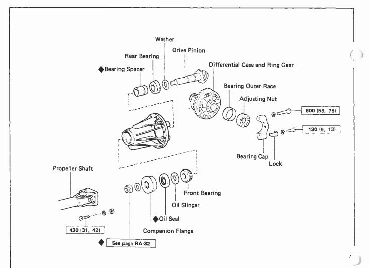
kg-cm (ft-lb, N-m) : Tightening torque
